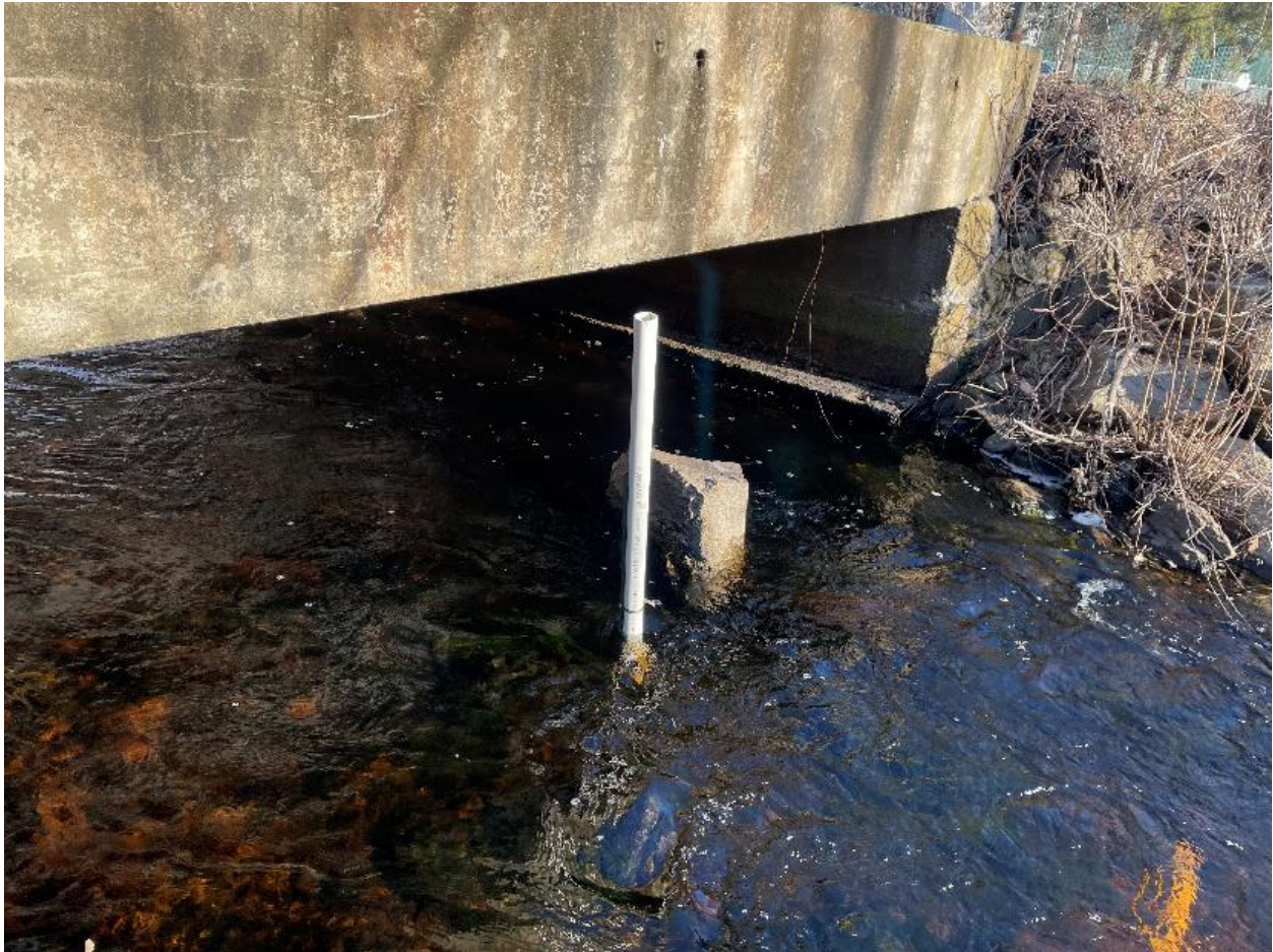
Figure 19. Water level monitoring well at the Pond Street crossing (Photo date: March 23, 2022).
