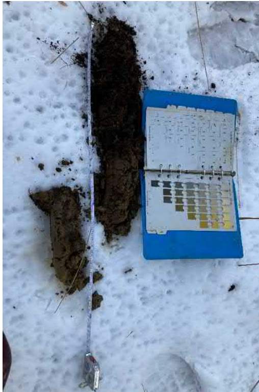
Photo 13 Soil pedon from STP4 within BVW from top to ~18" depth showing ~5" top layer of decomposed organics (1/17/23)
