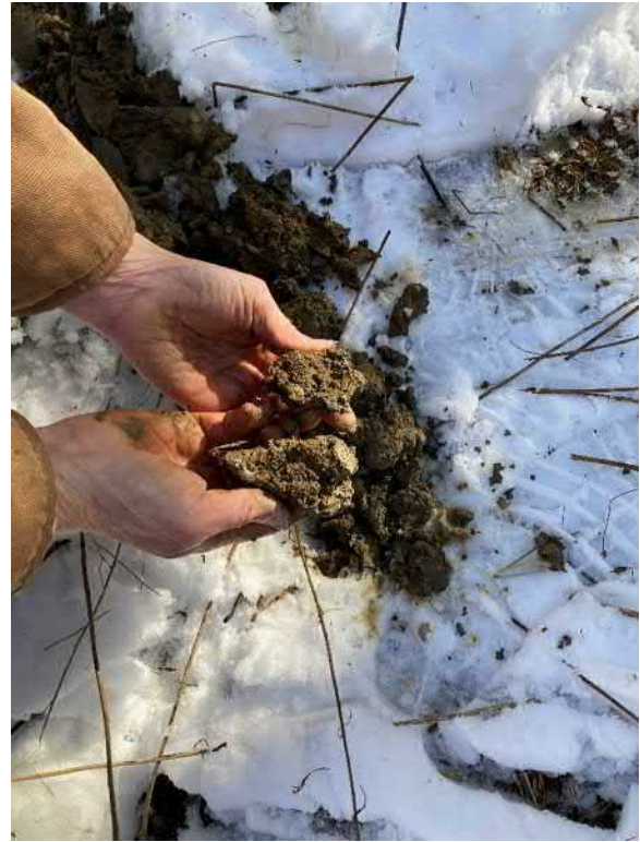
Photo 1 STP1 in easterly proposed wetland replication area; redoxymorphic features and saturation evident at ~20" from surface (including 1" O organic layer); note sheen on pedon and wet silt on hand) (1/17/23)
