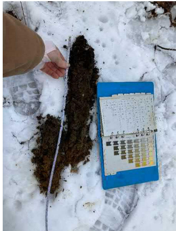
Photo 11 View of STP3 within proposed wetland replication area; approx. 2" organic layer [NOTE: pedon somewhat loose, so taped measurement appears as ~3"; refusal reached at ~18" below top of organic layer] (1/17/23)
